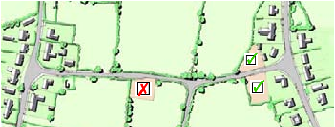
Site selection should respect the local settlement pattern and avoid infilling between existing building clusters
